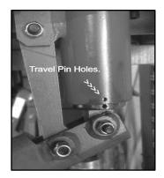
5. Remove the two manual pump linkage bolts from the lower section of the pump and remove the handle and linkage then put aside.
