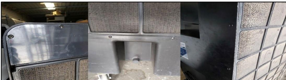
4. Use a water supply hose to manually fill the reservoir to the full level on the level indicator panel located at the rear of the unit below the air inlet panels, or if overfilled drain off the excess water to the correct full level.
