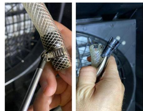
5. Fit the water supply hose to the new elbow.
