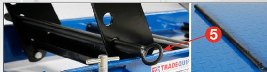
Raise to the desired height then insert the pin and operate the hydraulic release to take load onto the locking device assembly.
