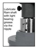
**Important:** Dirt is the greatest single cause of failure in hydraulic units. Keep the transmission lifter clean and well lubricated to prevent foreign matter from entering the system. If the Transmission Lifter has been exposed to rain, snow, sand, or grit it must be cleaned before it is stored or used.
