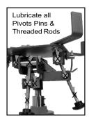
Periodically grease the ram shaft divider with a light bearing grease via the grease nipple provided.
