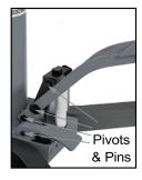
Wheel axles and Castor ball races should be lubricated with a Light Bearing Grease or 30/40W Machine Oil to ensure long life and prevent premature wear.
