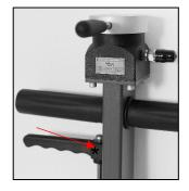
5. Regularly wind the screw extension to full length, clean with a suitable degreaser and apply a light bearing grease to ensure smooth operation when in use.
