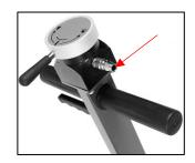
2. Rear "non load bearing wheels" and axles should be lubricated with a Light Bearing Grease or 30/40W Machine Oil to ensure long life, prevent premature wear and provide smooth rotation.
